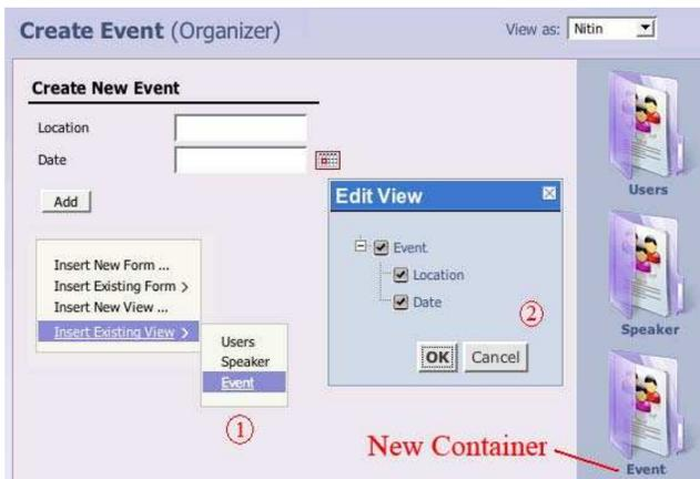
Figure 4: Adding a table to show existing events. The resulting table is shown in Figure 5.
