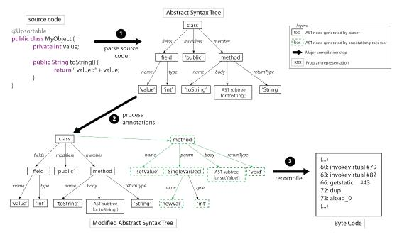
Figure 2: Upsortable Abstract Syntax Tree modifications at annotation processing time.
