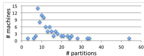
Figure 8: In a 128-machines cluster, GraphX does not balance number of partitions (1200) evenly to machines. A balanced distribution of workload would assign  $1200/128 = 9.4$  partitions to each machine. However, one machine has 54 partitions.
