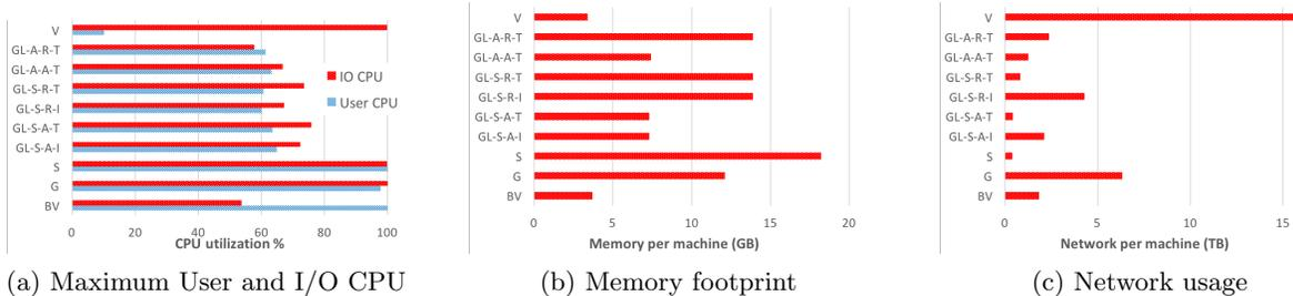
Figure 10: Understanding how Vertica use its computing resources in comparison to other systems. All results were collected while computing 55 iterations of PageRank for the UK0705 dataset using a cluster of 64 machines.
