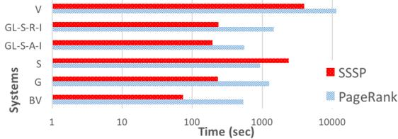
Figure 9: Computing SSSP (116 iterations) and 55 iterations of PageRank for the UK dataset using a cluster of 32 machines.
