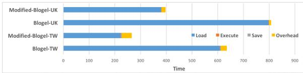
Figure 3: Performance of modified-Blugel in computing WCC using a cluster of 16 machines, without HDFS overhead between partitioning and workload execution. The load time, which represents data reading, partitioning, and shuffling before execution, has been significantly reduced.
