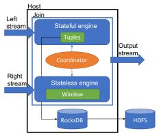
Figure 5: The join operator overview.
