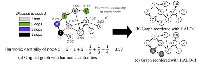
Figure 4: Graph reordering with HALO. HALO-I labels the nodes in decreasing order of centralities. HALO-II additionally labels the neighbours of nodes before moving to the next centrality score.
