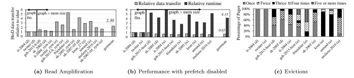
Figure 3: BFS performance characteristics on a Titan Xp GPU with UVM. (a) Average read amplification of 2.3x; (b) When the prefetcher is disabled, performance suffers severely despite a reduction in data transfer volume; (c) Distribution of the number of times the same pages are fetched from the host to device due to evictions
