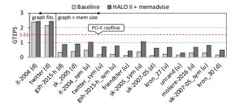
Figure 13: Overall performance after combining HALO-II reordering and the read-only memadyise hint
