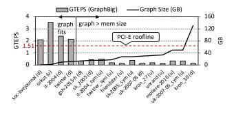
Figure 1: BFS performance measured in billions of Traversed Edges per Second (GTEPS) on a Titan Xp GPU
