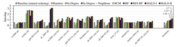
Figure 7: Multi-source BFS performance for different graph orderings relative to natural ordering on a Titan Xp GPU. Each kernel does a BFS from 10 random sources at the same time.
