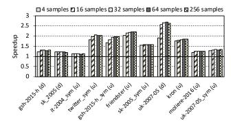
Figure 11: Sensitivity to the number of samples used in HALO-II. Performance saturates around 32 samples.
