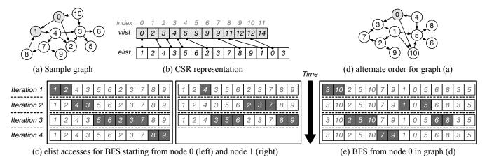
Figure 2: (a) A sample graph, (b) its CSR representation, (c) memory access pattern in elist for BFS from two different sources; (d) an alternate order for the graph, and (e) access pattern in the alternate order for traversal from node 0
