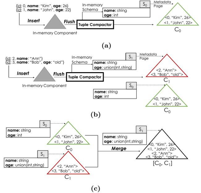
Figure 8: (a) Flushing the first component  $C_0$  (b) Flushing the second component  $C_1$  (c) Merging the two components  $C_0$  and  $C_1$  into the new component  $[C_0, C_1]$
