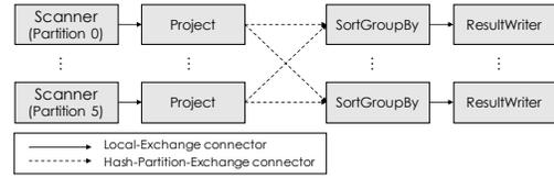
**Figure 5:** A compiled Hyracks job for the query in Figure 2
