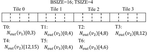
**Figure 5: Workload balance of tile-based residue push over three frontiers in a block with 16 threads.**
