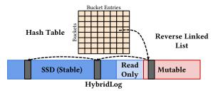
Figure 2: FASTER's HybridLog spans memory and SSD.
