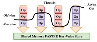
Figure 3: Asynchronous cuts in FASTER.
