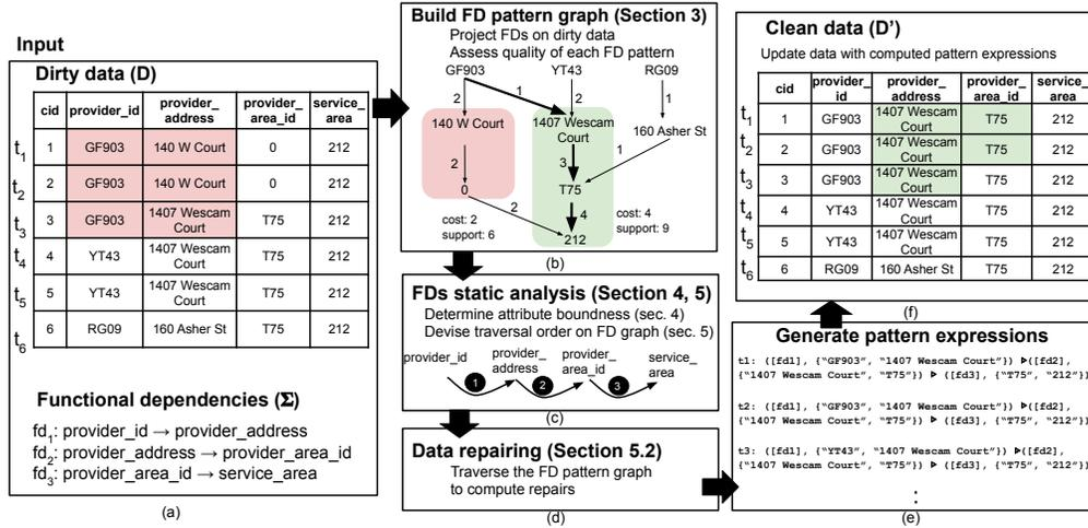
Figure 2: *Horizon* at a glance. (b) *Horizon* computes the FD pattern graph. (c) Performs static analysis on the FDs to devise a traversal order of the graph in Step (b). (d) Repairs the input tuples and presents the results to the user in (f) (e)
