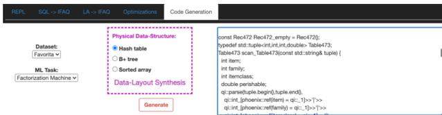
Figure 4: Screenshots of the IFAQ web user interface for code generation. Users can choose different data-layout options, and inspect the generated C++ code.
