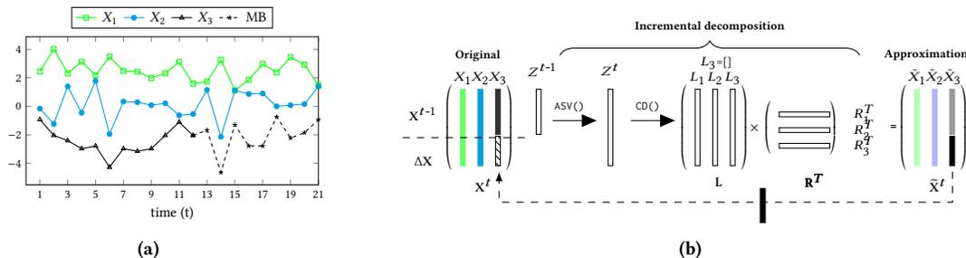
**Figure 1: Graphical illustration of the recovery of the missing block (MB) in  $X_3$  using ORBITS. (a) A plot of three input time series  $X_1$ ,  $X_2$  and  $X_3$  with a missing block represented by a dashed line at  $13 \leq t \leq 21$ . (b) ORBITS’s recovery, where CD decomposes the original data, exposing the matrix rank with dimensions  $L_1$ ,  $L_2$  and  $L_3$ .**
