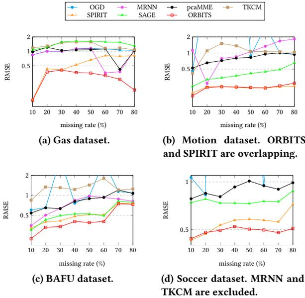
**Figure 5: Accuracy comparison with increasing missing block size.**
