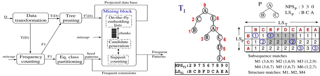
Figure 2: (a) Framework of our MCT algorithm (b) Example database tree, pattern, R-Matrix
