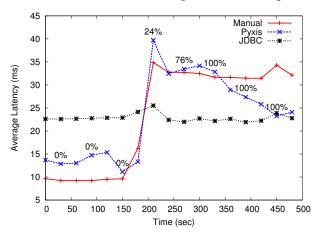
Figure 11: TPC-C performance results with dynamic switching
