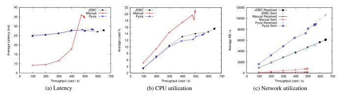
Figure 10: TPC-C experiment results on 3-core database server
