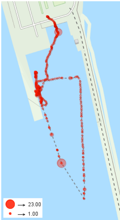
Figure 1: Analysis of the regularity of the position recording. The lengths of the time intervals between the recorded positions are represented by proportional sizes of circle symbols. The largest circle correspond to a time gap of 23 seconds, whereas the regular interval length is 1 second.
