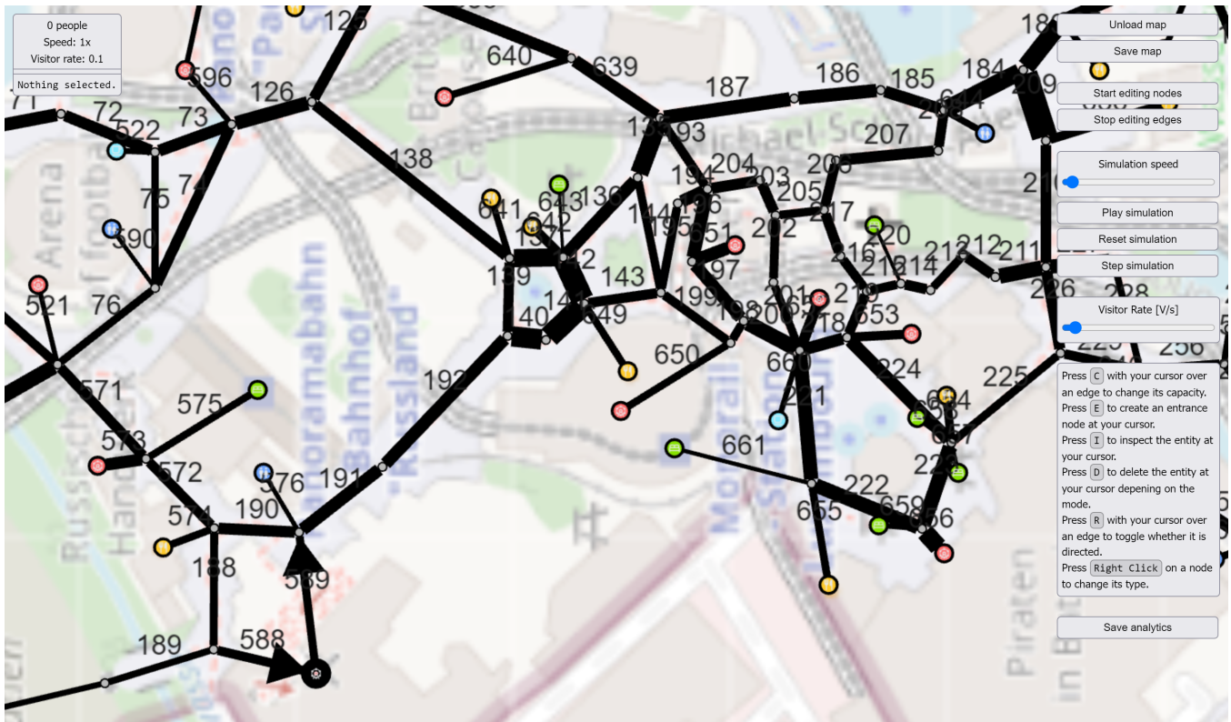
Figure 3: The graphical editor in XCrowd. Users can create and modify graph networks based on a reference background image, even with the simulation still running.
